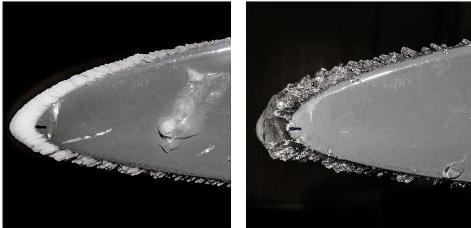
*Fig. 1: Rime ice (left) and glaze ice (right) accretions on a UAS airfoil from an icing wind tunnel test.*
