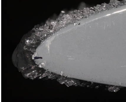
Figure 3: Clear ice accretion on a UAV airfoil from icing wind tunnel experiments.
