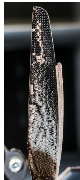
Figure 5: Ice shedding removed ice on the outer span of the propeller.
