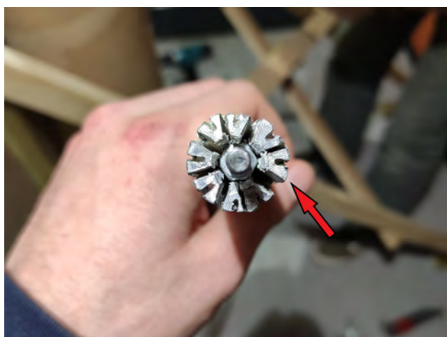
Fig. 4.11.: In axe direction view of the aluminium rod dissembled from the wing. The twisted part is indicated with the red arrow.
