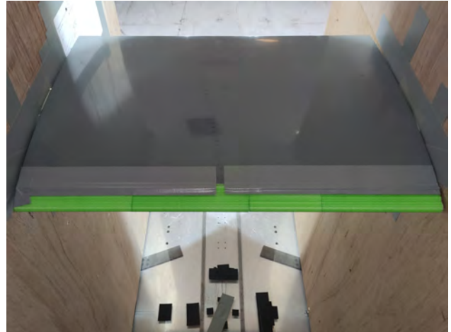
Fig. 2.8.: Artificial 3D-printed ice shape mounted at the leading edge of the wing with the aid of duct tape and spared out pressure holes in the middle of the wing.
