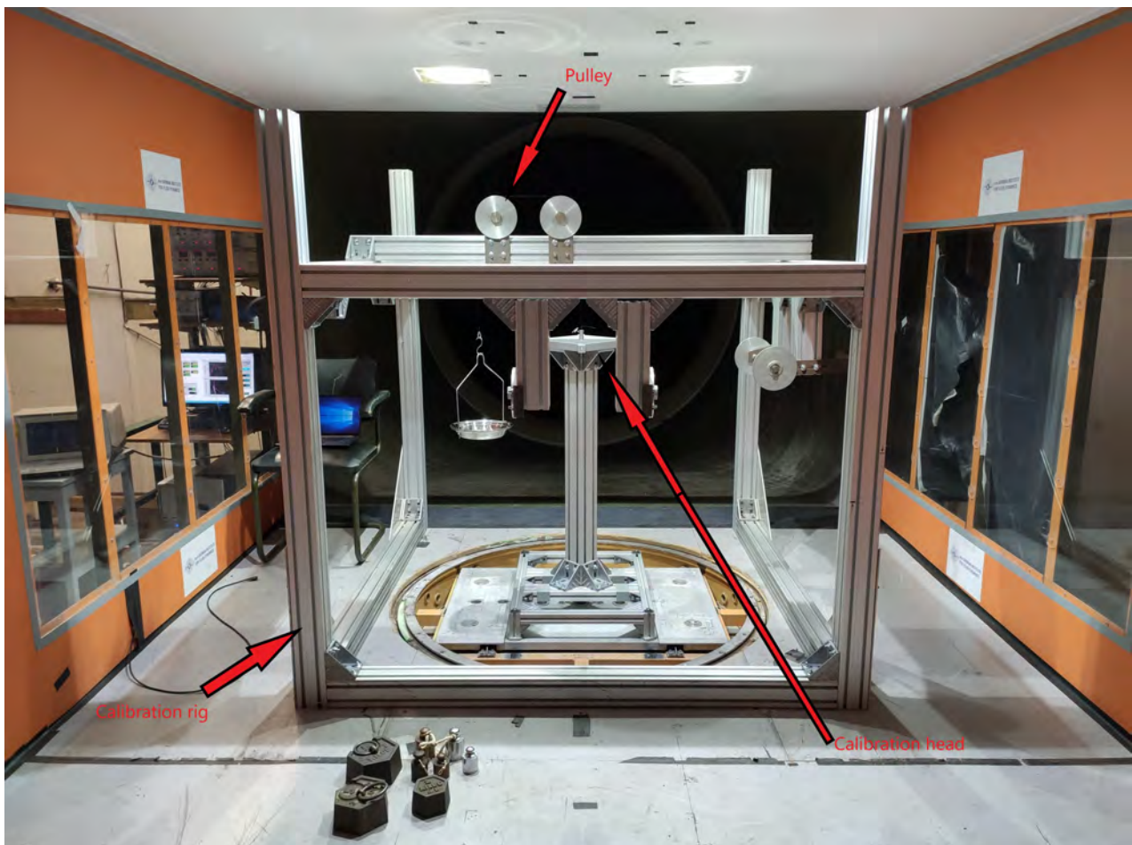
Fig. 2.10.: In flow direction view of the calibration rig mounted around the calibration head. The current setup represents the positive lift force imposing configuration with one pulley orientated with its edge directly above the centre of the calibration head, ensuring the hooked cable to be normal to the head's virtual plane.
