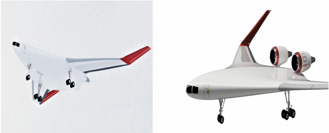
Figure 7: Blended Wing Body concept design. Source: [6]
