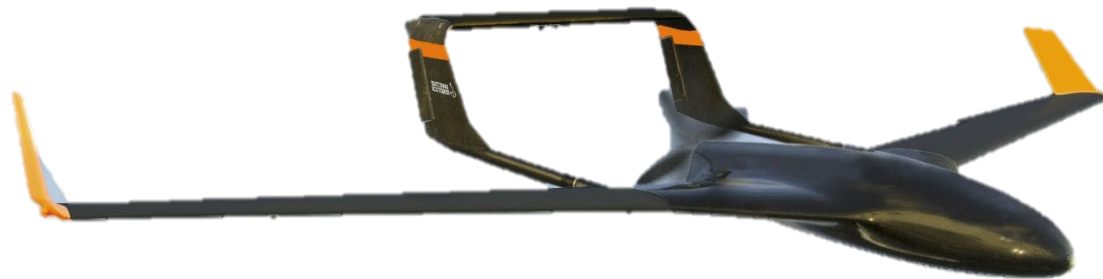
Maritime Robotics PX 31 Wingspan: 3.2 m Payload: 3 kg
