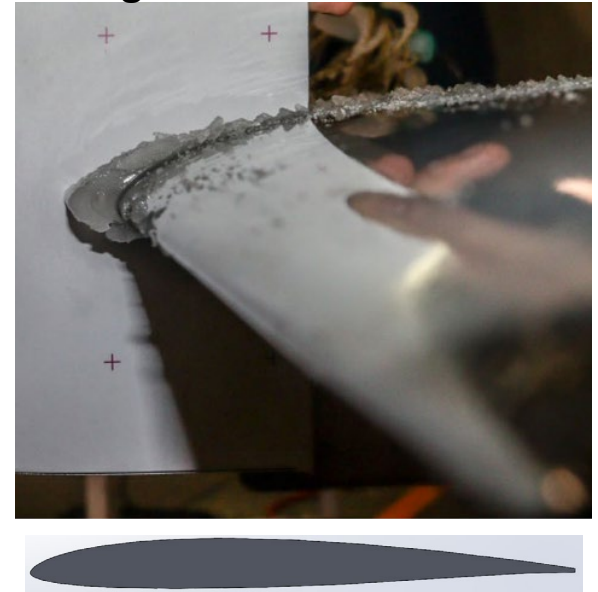
Case 3: RG-15 Low Speed Icing
