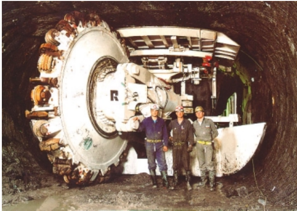
Figur 3.20 Mobile miner fra The Robbins Company.
