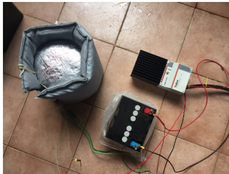
A small PV panel can over time accumulate cooking energy in a heat storage
