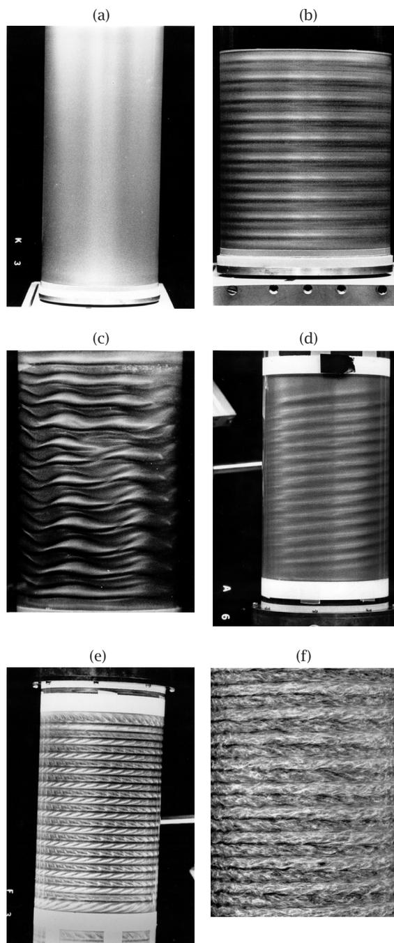
Figure 3 Some of the numerous flow patterns in the Taylor-Couette system: (a) Couette flow; (b) Taylor vortices; (c) wavy vortices; (d) spiral vortices; (e) twisted vortices; and (f) turbulent vortices. Source: Andereck et al. (1986).
