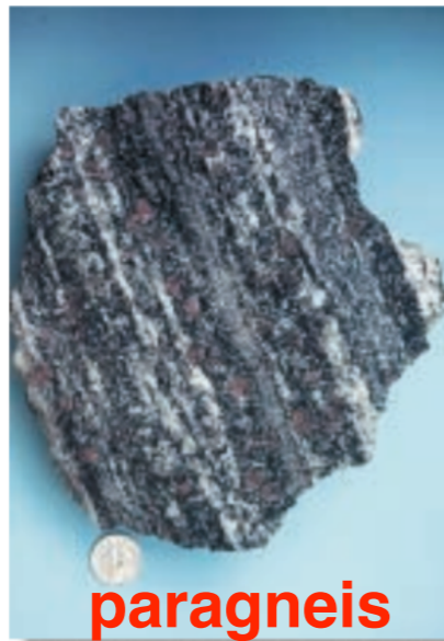
FIGURE 8.1 (a) Hand specimens of red shale, consisting of clay flakes, quartz, and iron oxide (hematite). (b) Hand specimen of metamorphic rock (gneiss) containing biotite, quartz, feldspar, and bright purple garnets. A rock similar to the shale could have been the protolith of this gneiss. This hand specimen is about 10 cm wide. (c) This thin section of a Devonian limestone shows that the rock consists of small fossil shells and shell fragments that have been cemented together. The field of view is about 3 mm. (d) This thin section of marble shows how new crystals of metamorphic calcite grew to form an interlocking texture. This photo is taken with polarized light; the color and darkness of an individual grain depends on its orientation with respect to the light waves. (e) Granite has randomly oriented grains. (f) Metamorphosed granite has flattened and aligned grains.
