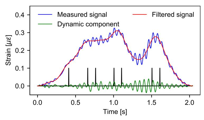
Kalin, Anžlin, Kreslin, Žnidarič. *Measurements of Bridge Dynamic Amplification Factor Using Bridge Weigh-in-Motion Data*, accpt. for publ. in Structure & Infrastructure Engineering
