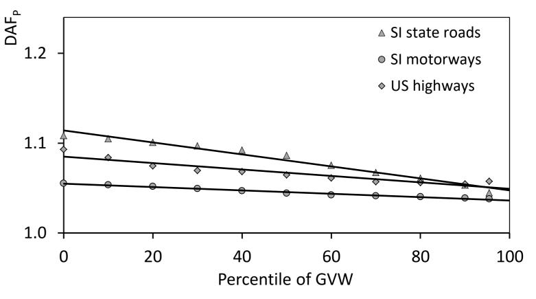
Kalin, Anžlin, Kreslin, Žnidarič. *Measurements of Bridge Dynamic Amplification Factor Using Bridge Weigh-in-Motion Data*, acc. for publ. in Structure & Infrastructure Engineering
