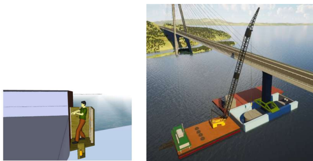
Fig. 2 Repair of a steel pontoon using a cofferdam (left) and drydock (right) to facilitate a dry atmosphere during repair.
