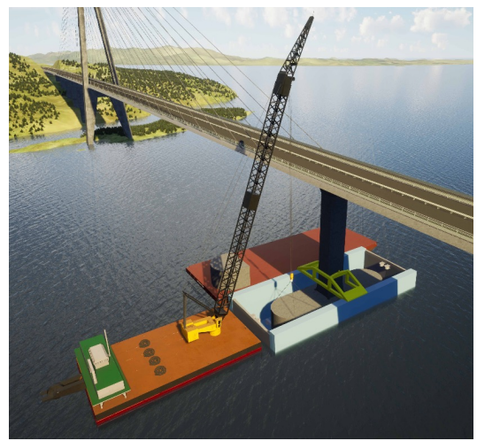
Repair scenario - pontoon carried by a drydock
