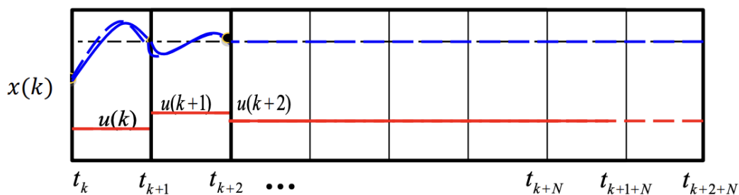
Figure 3: Illustration of the state trajectory x and input sequence u at every sampling instant k over the prediction horizon. The NMPC only provides the first element of the input sequence to the Plant
