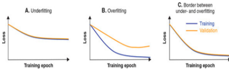
Figure 3.2: The figure shows three simplified plots of validation and training loss during training. Case A shows underfitting, where the training and validation loss ceases to decrease after a short period, remaining at a high value. Case B shows overfitting, where the validation loss starts to increase, while training loss decreases further. Case C shows a "just right" fitted model, where training and validation loss decreases somewhat simultaneously throughout the training period [25].
