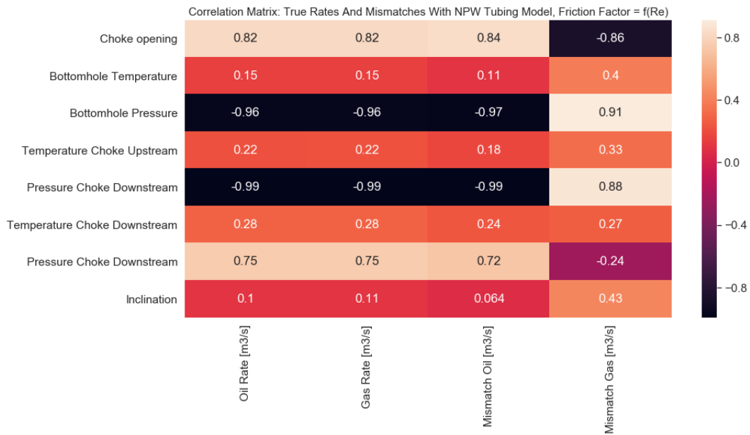
Figure 39: Pearson correlation matrix for true rates and mismatches calculated with the NPW tubing model.
