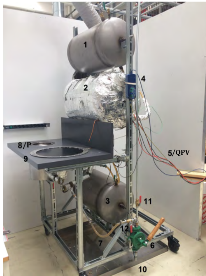
Figure 2.1: Picture of the system assembled at the NTNU laboratory. The equivalent system in Arusha contains a larger cooker (8) and no frying pan (9). The picture and table 2.1 below are retrieved from reference [5].
