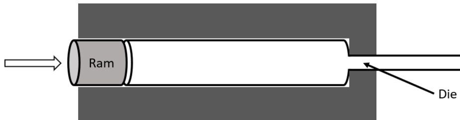
Figure 2.3: Illustration of direct extrusion.
