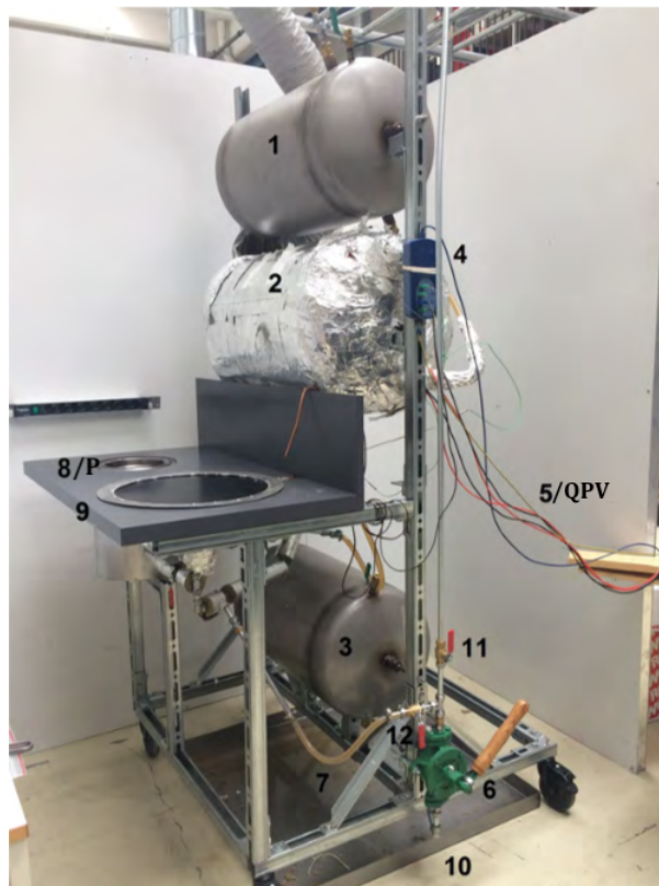
Figure 3.1: Overview of the system at NTNU, with labels described in table 3.1. The prototype in Arusha has replaced the frying pan (9) with a larger cooker (8). The picture and table 3.1 are reproduced from reference [8].
