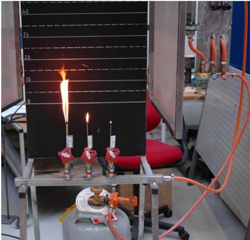
In this exercise you are going to determine different characteristic quantities for a vertical flame. The fuel is propane and three different nozzles (diameters) are available. The velocity of the fuel flow can be estimated from the flow rate, which is measured by a rotameter.
