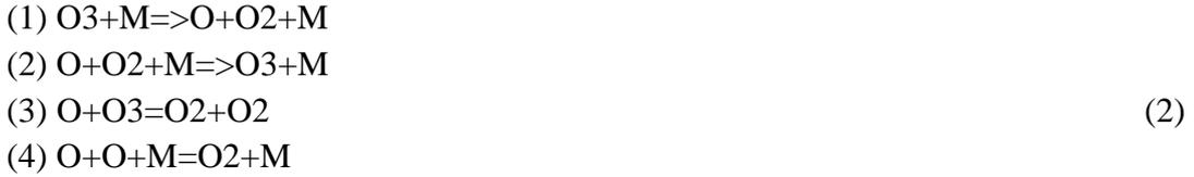
Reaction 1 is an endothermic reaction that produces the radical O necessary for the combustion to occur. Reaction 3 is responsible for the most of the oxidation of the radical. The Arrhenius coefficients are the same used by [10].
