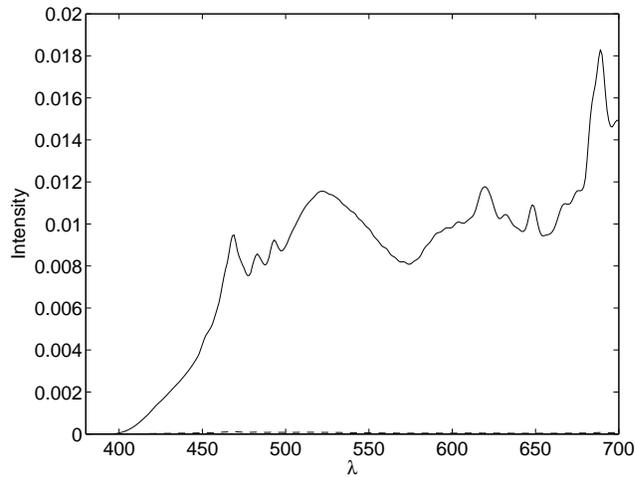
(b) Example white spectrum obtained by opening all pixels of the window on the LCD panel. The dashed line shows the black spectrum for comparison.
