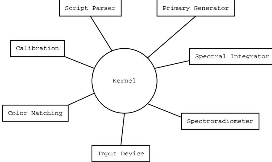
**Figure 3.** Overall architecture for the executive software for the spectral integrator. See Section 3.1 for details.
