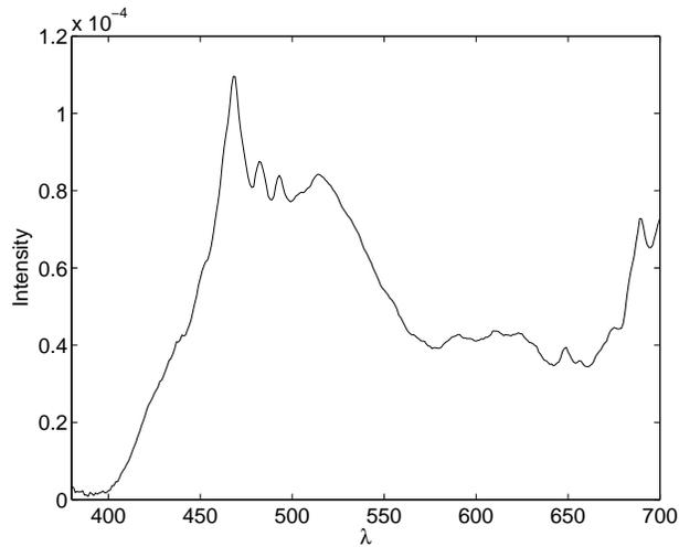
(a) Example black spectrum obtained by closing all pixels of the window on the LCD panel.
