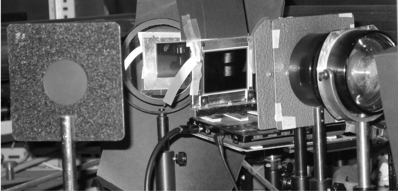
**Figure 2.** A detailed view of the spectral integrator prototype at UiO (from right) a lens, the transmissive LCD panel with two spectra, a mirror, and the dispersing plate onto which the resulting colored light is projected.
