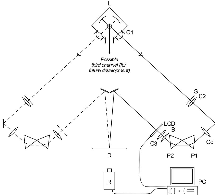
**Figure 1.** Principal sketch of the spectral integrator. (L) lamphouse, (C1)–(C3) condensor lenses, (S) water-cooled slit, (Co) collimator, (P1)–(P2) dispersing prisms, (LCD) transmissive LCD panel, (D) dispersing plate, (B) biprism (optional), (R) spectroradiometer, (PC) administrative PC unit.
