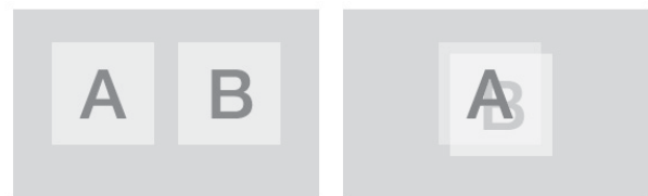
Figure 1. Experimental setup. On the left a traditional pair comparison setup with two reproductions (A and B) next to each other, which was used in the work by Farup et al. [1]. On the right the setup used in this work, where the images are placed on “top” of each other at the same location and the observers could flip between them.
