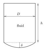
The relevant physical quantities in this problem are the geometry of the vessel (parametrized by d, D and  $\delta$ ), the density  $\rho$  and the height h of the liquid which determine the action of the gravity and the modulus of elasticity E which gives a relation between stress and deformation (it relates somehow the pressure and  $\delta$ ).
