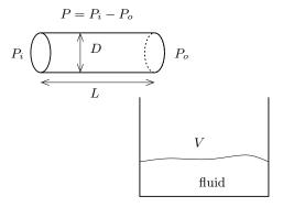
The time required to fill in the vessel depends directly on the flow coming out of the pipe. The flow depends on the diameter of the pipe (D) and on the velocity of the liquid. The striving force in this experiment is the pressure (we assume gravity is not involved) which act through its gradient. Therefore  $P = P_i - P_o$  and L must be considered as relevant variables. Roughly speaking, the viscosity  $\mu$  determines the fluid response to a given excitation and it must be taken into
