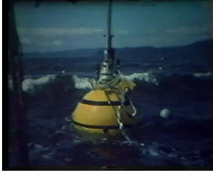
Phase-controlled power-buoy model (type E) under test in the Trondheim Fjord, 1983. Video clip [also on http://folk.ntnu.no/falnes/w_e/ .]
