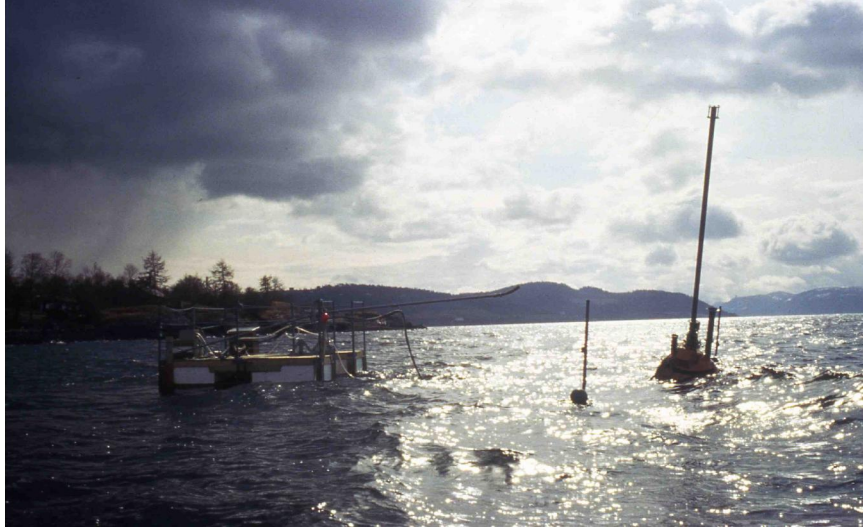
Budal's phase-controlled power buoy model (type N2) at the test site in Trondheimsfjorden.
