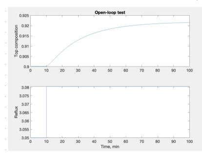
2. Using the plot obtained, find a 1st order transfer function model  $\left(G(s) = k \frac{e^{-\theta s}}{\tau s + 1}\right)$ from u to y (where  $y \equiv x_D$ ). (Hint, the steady-state gain is  $k = \frac{\Delta y}{\Delta u}$  at steady
