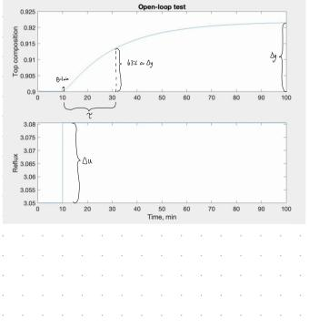
3. Tune a PI controller using SIMC rule (Eq. 1 - must be memorized!. Try  $\tau_c=3$  min,  $\tau_c = 1$  min and  $\tau_c = 0.5$  min and simulate for disturbances and setpoint changes. Print the results and give the parameters obtained. Notice that a measurement delay of 1 min has been included in the feedback loop, so  $\theta = 1$  min.
