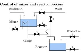
Figure 1: Control of mixer/reactor process
