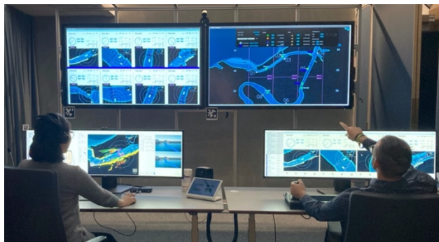
Figure 11: The NTNU Shore Control Lab with a prototype of an HMI giving situation awareness and automation transparency to operators.
