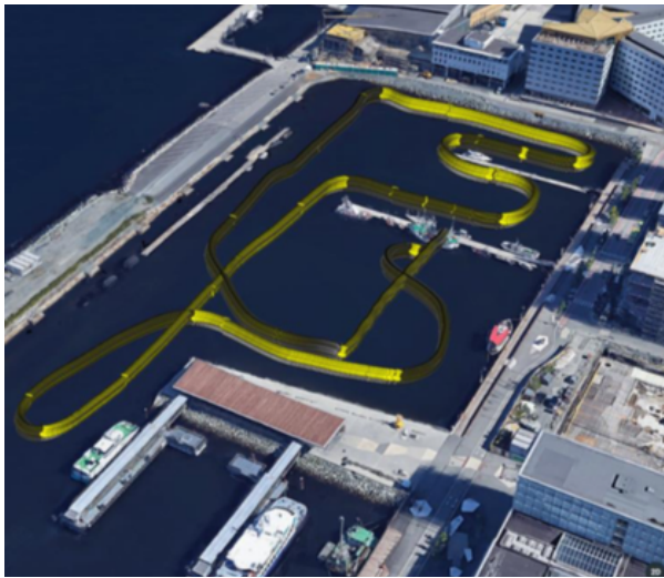
Figure 9: Trajectory of milliAmpere1 during SLAM experiments in Brattørabassenget (left), together with experimental results (right) [22].
