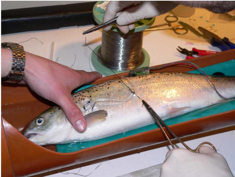
**Figure 5: The full installation of an opercular differential pressure tag. This tag falls in a category of its own, as it is only a prototype for laboratory experiments, and utilizes a hard-wire transfer of sensor signals.**
