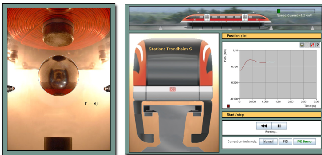
Figure 4 Magnetic levitation is visualised in two different disguises. To the left a magnetic ball balances in an electromagnetic field. To the right a magnetic levitation train is used in an educational game.
