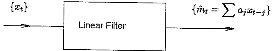
Figure 1-20 Smoothing with a low-pass linear filter.
