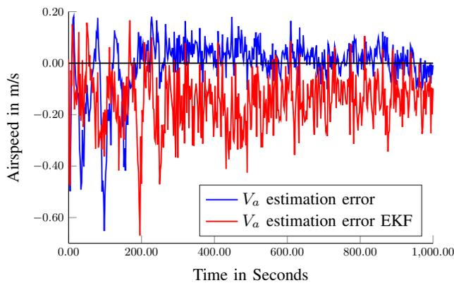
Fig. 8: Airspeed estimation error,  $RMSE = 0.08m/s$ ,  $RMSE_{EKF} = 0.18m/s$
