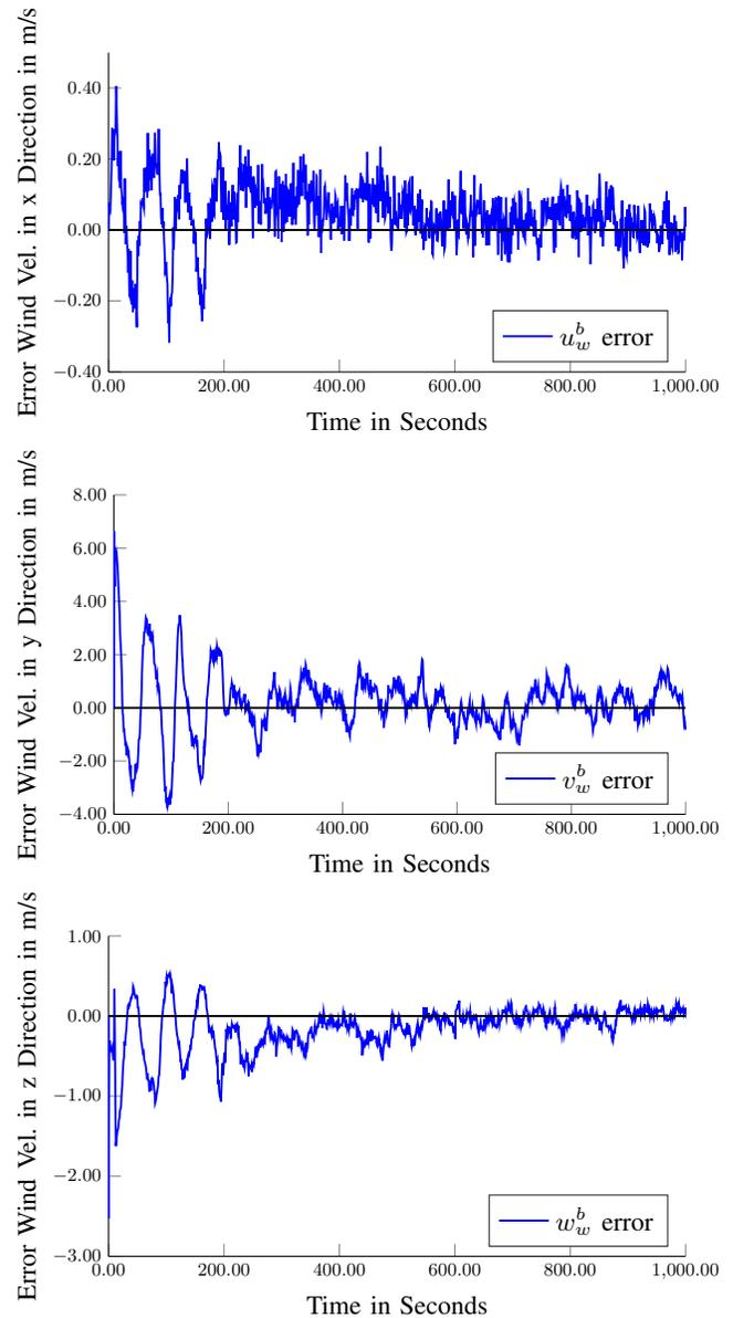
Fig. 7: Wind velocity estimation error in body frame
