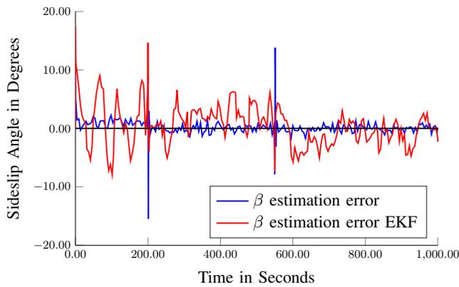
Fig. 10: Sideslip angle estimation error  $RMSE = 1.06^\circ$ ,  $RMSE_{EKF} = 9.34^\circ$
