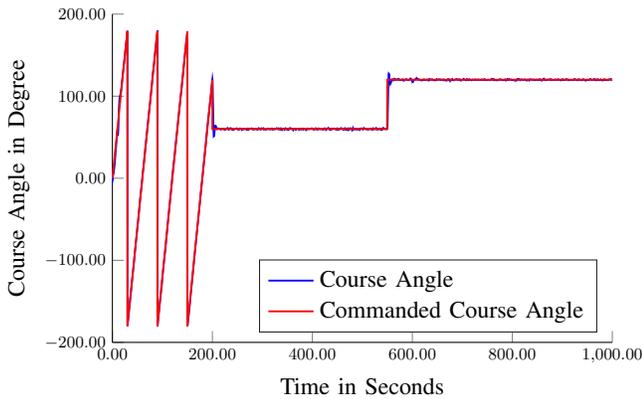
Fig. 4: Commanded and resulting course angle of the UAV
