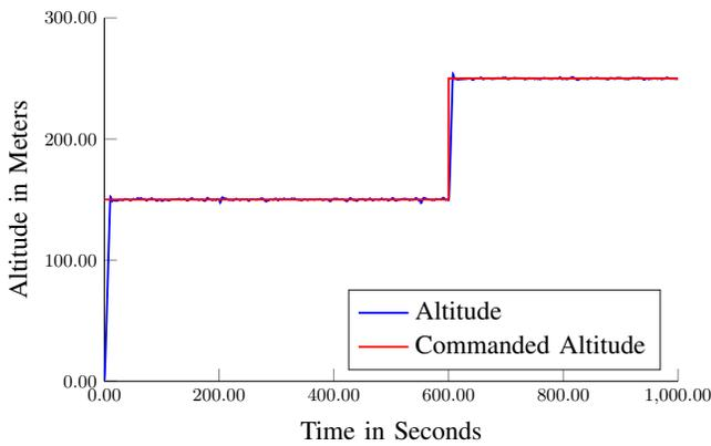
Fig. 3: Commanded and resulting altitude of the UAV
