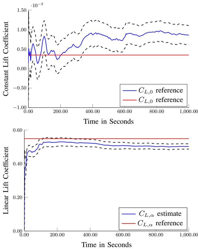
Fig. 6: Estimates of static and linear lift coefficient for  $c = 20$ , dashed black lines indicate  $3\sigma$  interval
