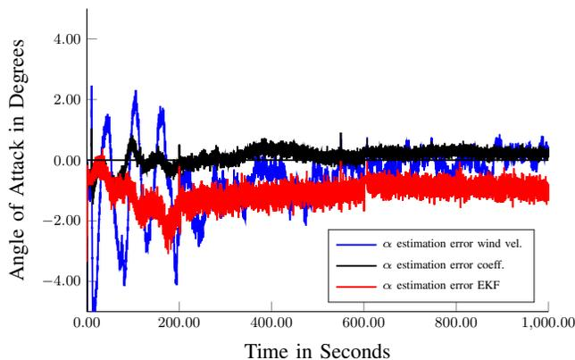
Fig. 9: Comparison of Angle of Attack calculation methods,  $RMSE_w = 0.93^\circ$ ,  $RMSE_c = 0.25^\circ$ ,  $RMSE_{EKF} = 1.16^\circ$
