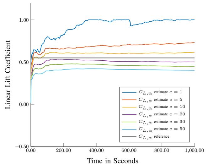
Fig. 5: Estimates of linear lift coefficient for different values of  $c$
