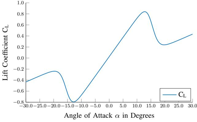
Fig. 2: Nonlinear model of the lift coefficient
