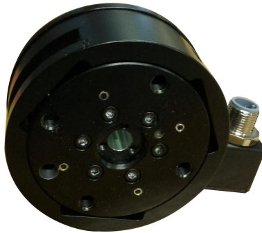
Figure 4.2.: The ATI Gamma netft F/T sensor which measures all six components of force and torque, i.e., F_x , F_y , F_z , n_x , n_y and n_z .
