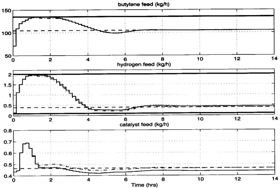
Figure 8.10: Closed-loop trajectories manipulated variables with back-off. Applied inputs (solid), reference inputs (dashed-dotted) and nominal target values (dashed).
