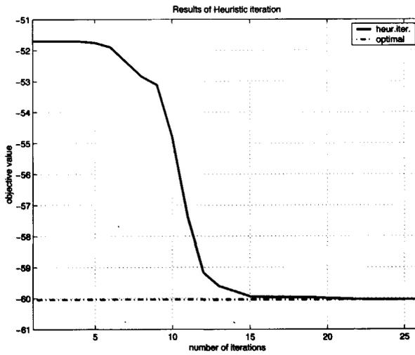
Figure 5.1: Optimal result for the distillation column. Dashed-dotted line: optimal value via conic solver, solid line: solution of heuristic iteration.
