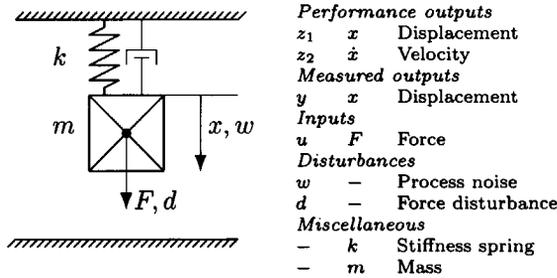
Figure 4.8: The mass-damper-spring example
