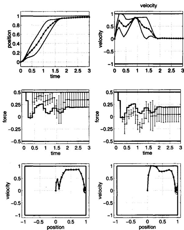
Figure 4.10: Optimal result for the bounded disturbance case with measurement noise.
