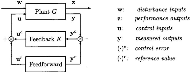
Figure 4.1: The generalized plant for predictive control
