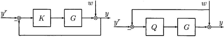
Figure 4.6: Direct design in  $K$  vs. analytical design in  $Q$ .
