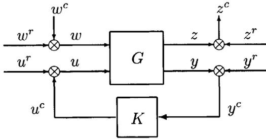
Figure 3.4: Interconnecting the generalized plant with the controller.
