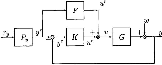
Figure 4.4: Classical 2 degrees-of-freedom feedback/feedforward design.  $G$ : open-loop plant,  $F$ : feedforward filter  $K$ : controller,  $P_y$ : pre-filter.
