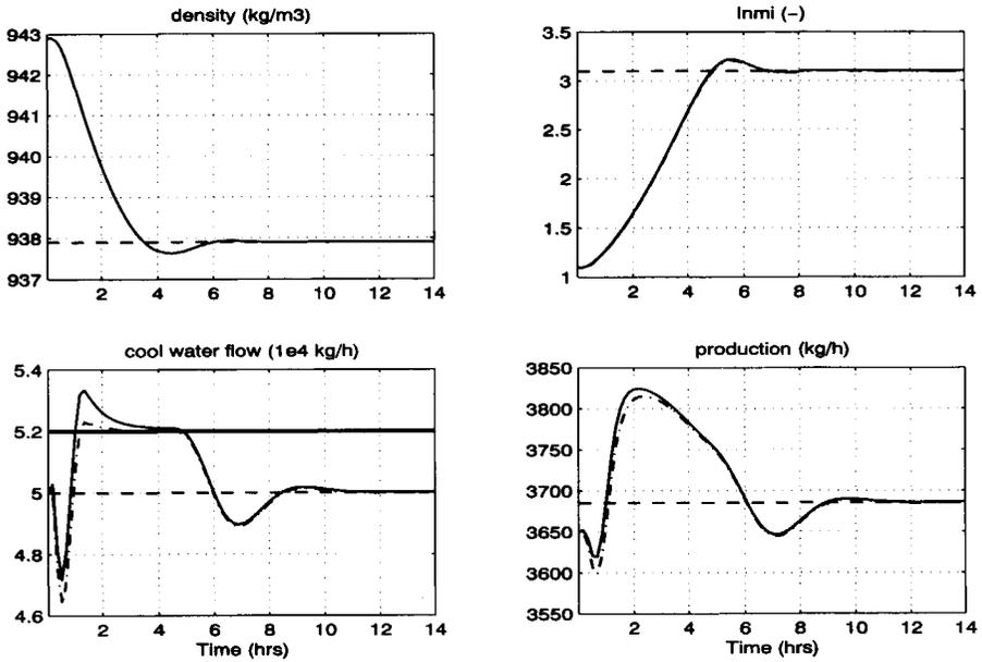
Figure 8.6: Closed-loop trajectories of controlled variables using EKF+LTV-MPC. Real performance (solid), estimated performance (dash-dotted), target performance (dashed).
