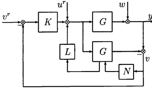
Figure 7.1: Innovations feedback with state-feedback; a closed-loop predictive alternative to open-loop internal model control.
