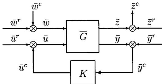
Figure 3.3: Interconnecting the generalized plant with the controller.
