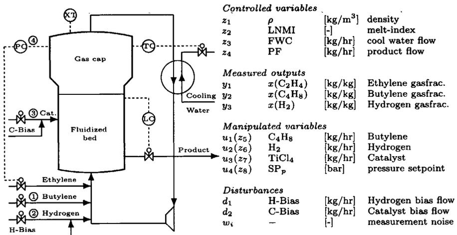
Figure 8.1: Process schematic of the fluidized bed reactor
