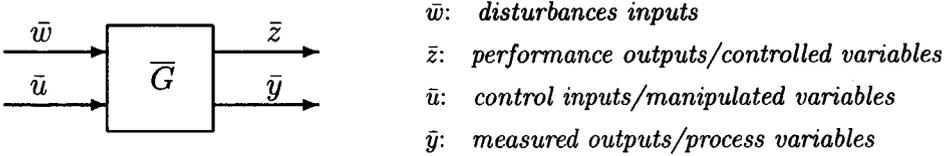
Figure 3.1: The input-output structure of a generalized plant.
