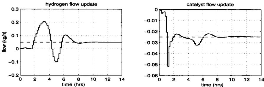
Figure 8.5: Bias compensation using EKF+LTV-MPC. Real values (solid), H-Bias (dashed), C-Bias (dashed).
