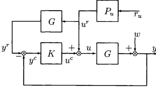
Figure 4.5: Predictive 2 degrees-of-freedom feedback/feedforward design.  $G$ : open-loop plant,  $K$ : controller,  $P_u$ : pre-filter (dynamic optimization).
