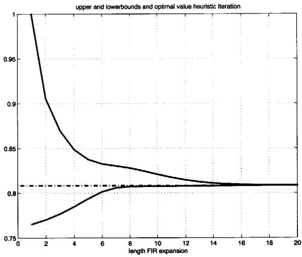
Figure 6.4: Result of upper and lower bound computation (*solid*) and the heuristic algorithm after 4 iterations, (*dash-dotted*).
