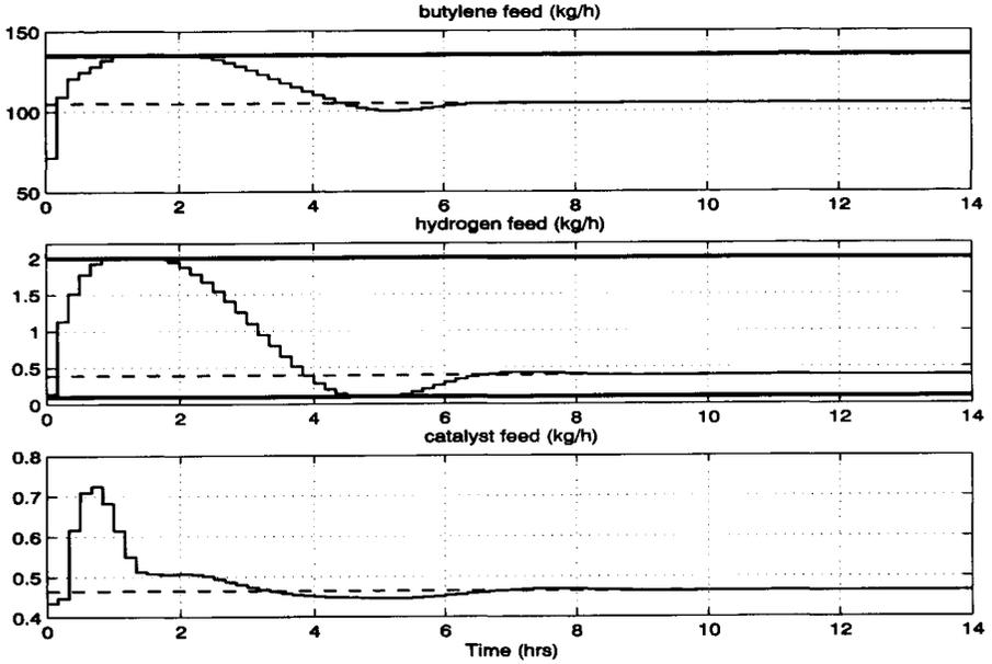
Figure 8.3: Open-loop trajectories of the control inputs. Applied inputs (solid) and nominal target inputs (dashed).
