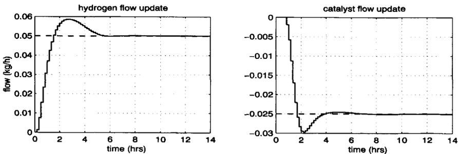
Figure 8.8: Bias compensation using the closed-loop predictive controller. Real values (solid), H-Bias (dashed), C-Bias (dashed).
