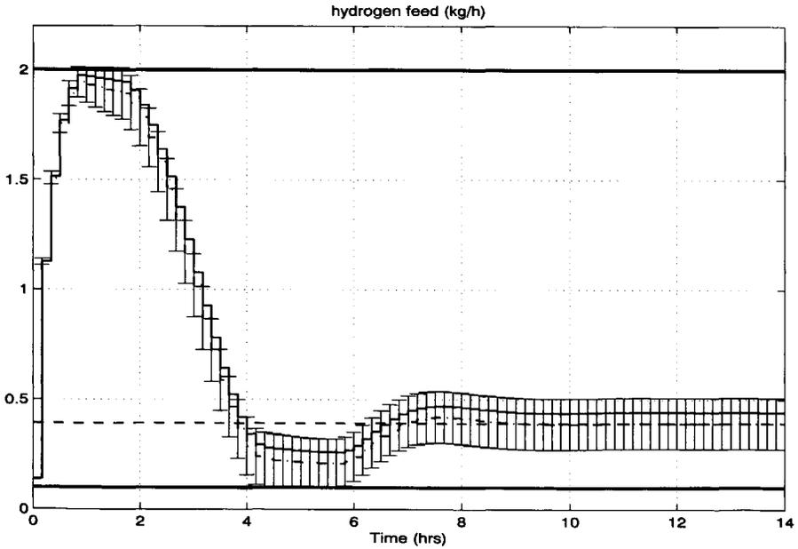
Figure 8.12: Close-up of closed-loop hydrogen feed flow. Applied (solid), reference (dashed-dotted) and nominal target value (dashed).
