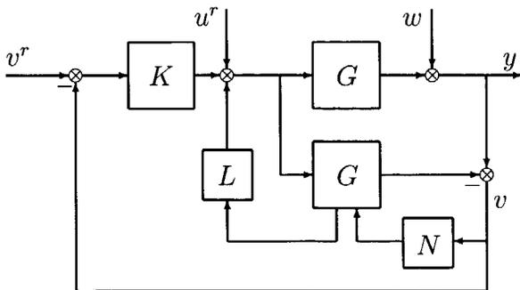
Figure 4.11: The Youla-Kučera parameterization via state and innovations feedback. A closed-loop predictive alternative to open-loop internal model control.
