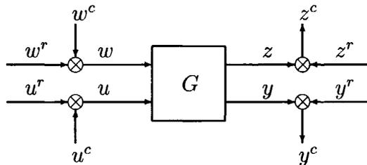
Figure 4.2: Generalized plant with reference signals.
