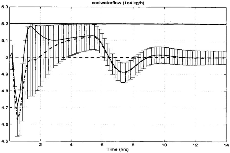
Figure 8.11: Close-up closed-loop cool water flow. Real (solid), reference (dash-dotted), target (dashed).
