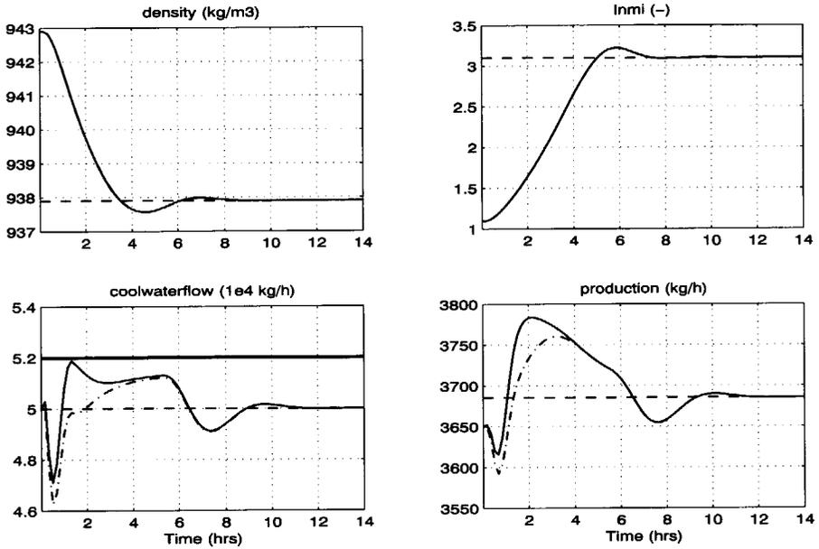
Figure 8.9: Closed-loop trajectories controlled variables with back-off. Real performance (solid), reference performance (dash-dotted), target performance (dashed).
