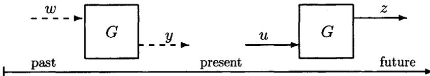
Figure 3.6: The classical decomposition of LQG control. The estimation problem considers disturbances and measured outputs only in past (dotted); the control law considers deterministic inputs and performance outputs only in future (solid).
