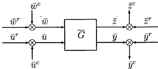
Figure 3.2: Adding reference signals to the generalized plant set-up.
