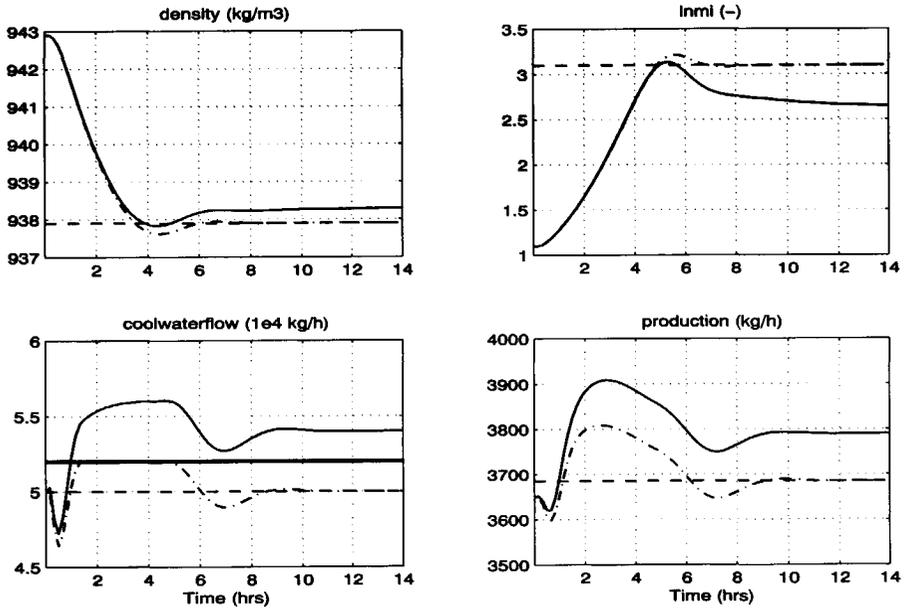
Figure 8.4: Open-loop trajectories of the controlled variables for the grade change. Real performance (solid), reference performance (dash-dotted), target performance grade B (dashed).
