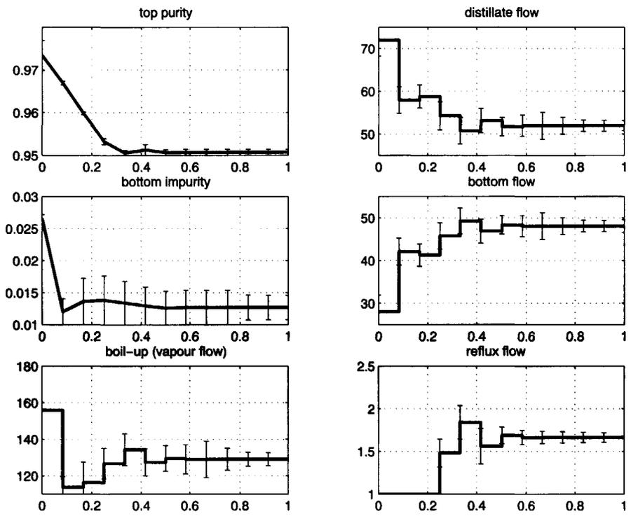
Figure 4.13: Optimal transition of column to new set-point. Solid-lines represent the reference feedforward trajectory. Error-bars represent uncertainty in the transition in closed-loop.
