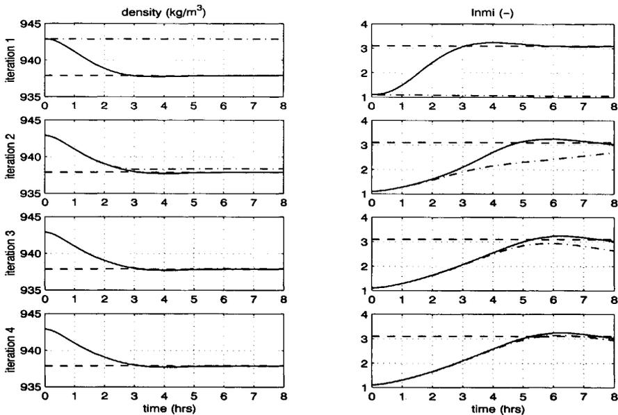
Figure 8.2: First four iterations in LTV method. Performance after optimization before simulation (solid), performance before optimization after simulation (dash-dotted), nominal target performance (solid).
