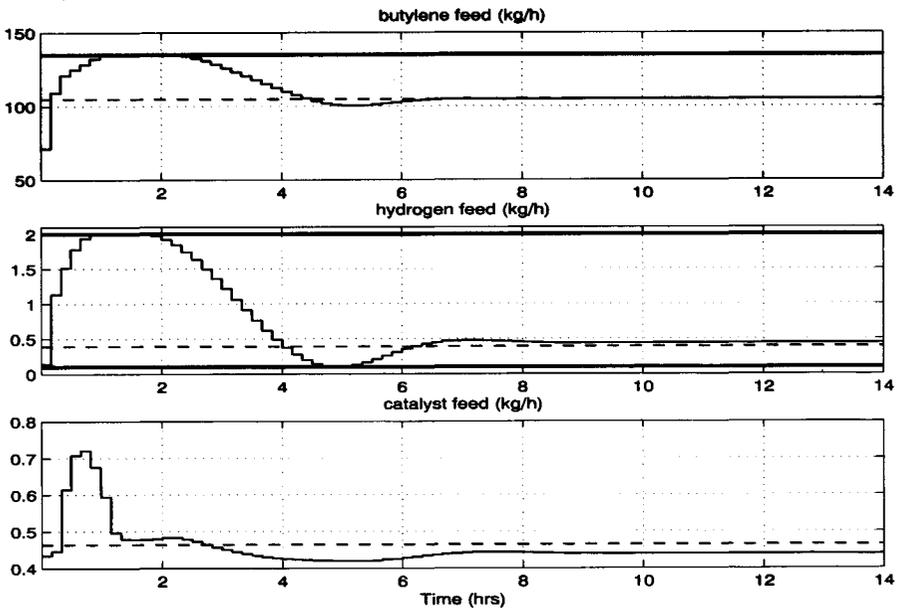
Figure 8.7: Closed-loop trajectories manipulated variables using EKF+LTV-MPC. Applied inputs (solid) and nominal target values (dashed).
