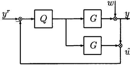
Figure 4.7: Internal Model Control.
