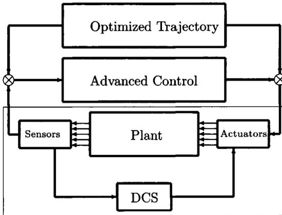
Figure 1.1: Constructive view on optimization and control.
