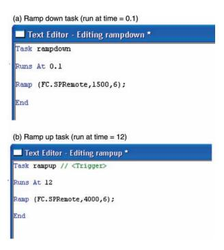
**Figure 15.6** Tasks for ramping set point of flow controller. (a) Ramp down task (run at time = 0.1). (b) Ramp up task (run at time = 12).
