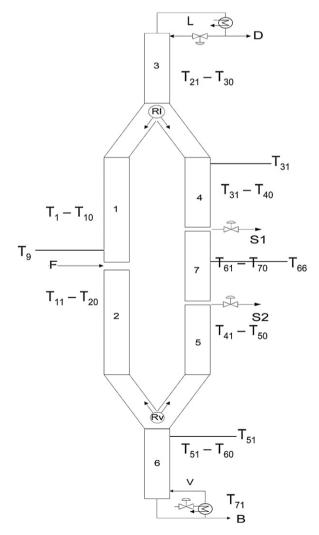
Fig. 8. Kaibel distillation column with 7 sections.
