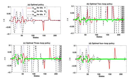
**Fig. 9.** Kaibel column state drift in the presence of disturbances in V,  $R_V$  and F, (a) optimal policy (minimum achievable state drift), (b) optimal two-loop policy, (c) optimal three-loop policy, (d) optimal four-loop policy. The effect of a measurement noise on state drift is shown with green +in subplots (b), (c) and (d).
