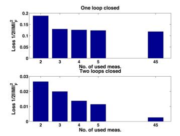
**Fig. 6.** Distillation case study: the reduction in loss in state drift vs number of used measurements. Top: loss with one loop closed, bottom: loss with two loops closed.
