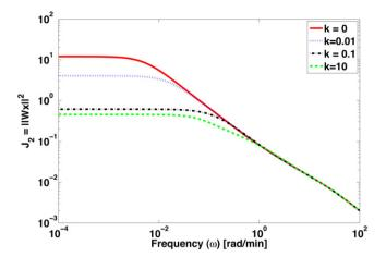
**Fig. 4.** State drift  $J_2$  for distillation column as a function of temperature controller gain k.
