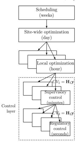
Fig. 1. Control system hierarchy for plantwide control in chemical plants [1].
