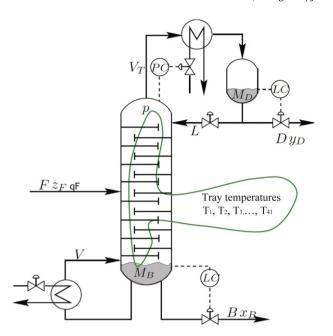
Fig. 3. Distillation column using LV-configuration.
