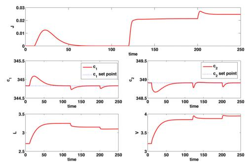
**Fig. 7.** Distillation case study: transient responses of state drift, J with two temperature loops closed ( $c_1 = T_{27}$ ,  $c_2 = T_{15}$ ) using inputs L, V for +20% disturbance in F at time 10 min, +20% disturbance in  $z_F$  at time 120 min and +10% disturbance in  $q_F$  at time 200 min.
