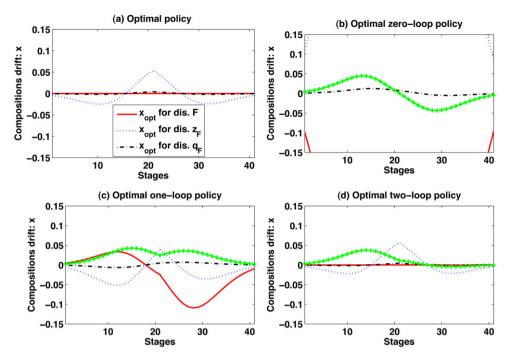
**Fig. 5.** Distillation column state drift in the presence of disturbances F,  $Z_F$ ,  $q_F$ : (a) optimal policy (minimum achievable state drift), (b) optimal zero-loop policy, (c) optimal one-loop policy, (d) optimal two-loop policy. The effect of a measurement noise on state drift is shown with green +in subplots (b), (c) and (d).
