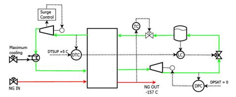
Fig. 5. Suggested control structure for the PRICO process. TC = Temperature controller, LC = level (active charge) controller, DTC =  $\Delta T$  controller and DPC =  $\Delta P$  controller.
