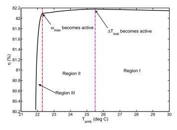
**Fig. 4.** Compressor efficiency at the optimal solution, as function of ambient temperature  $T_{amb}$  for  $F = F_{nominal}$ .
