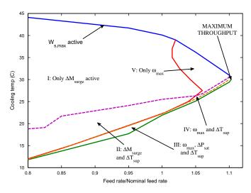
**Fig. 2.** Active constraint regions for the PRICO process, as function of feed flow rate F and ambient temperature  $T_{amb}$ .
