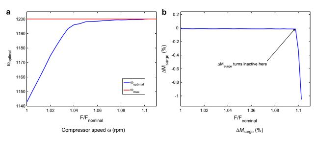
Fig. 3. Plots of optimal compressor speed ( $\omega$ ) and distance to surge ( $\Delta M_{surge}$ ) as function of  $F/F_{nominal}$  when going from Region I to Region V.
