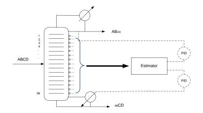
Figure 5: Schematic of the distillation process with estimator
