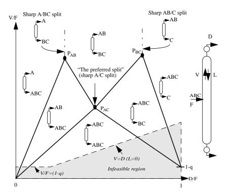
Figure 2.9: Regions of distributing feed components as function of V and D for a feed mixture with three components: ABC.  $P_{ij}$  represent minimum energy for sharp split between component i and j. For large vapour flow (above the top "saw-tooth"), only one component distribute. In the triangle below  $P_{AC}$ , all components distribute.
