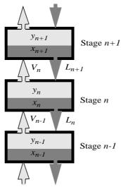
Figure 2.3: Distillation column section modelled as a set of connected equilibrium stages
