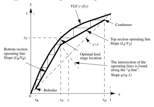
Figure 2.6: McCabe-Thiele Diagram with an optimally located feed.
