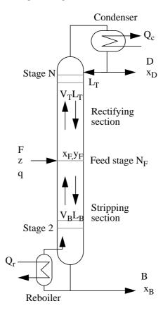
Figure 2.5: An ordinary continuous two-product distillation column
