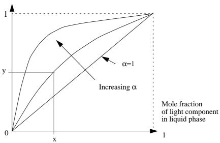
Figure 2.2: VLE for ideal binary mixture:  $y = \frac{\alpha x}{1 + (\alpha - 1)x}$
