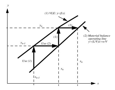
Figure 2.4: Combining the VLE and the operating line to compute mole fractions in a section of equilibrium stages.
