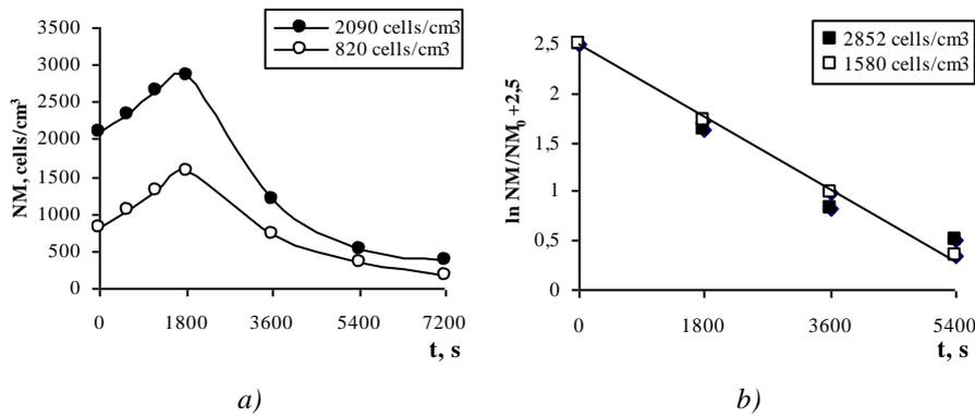
Figure 2: Effect of US action on the NM in the natural water during all process (a) and at the stage of microorganisms destruction (b). Conditions:  $T=298\pm 1K$ ,  $P=0.1MPa$ , US frequency of 22 kHz, power of 35 W.
