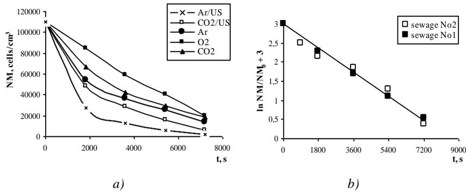
Figure 3: Effects of different gases and gas/US action on the NM in the sewage  $N_{o1}$  (a) and effect of  $O_2/US$  action on the NM in the sewage  $N_{o1}$  and  $N_{o2}$  (b). Conditions:  $T=298\pm 1K$ ,  $P=0.1MPa$ , US frequency of 22 kHz, power of 35 W.
