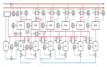
Fig. 1. Flow sheet of the drying section. Red lines indicate steam pipes, blue lines are condensate pipes and purple lines indicate mixed flow of steam and condensate
