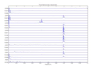
Fig. 3. Power spectra of the process measurements (PVs)
