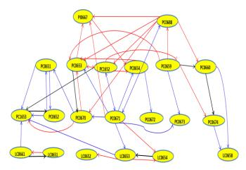
Fig. 7. Causal digraph based on the max PDC values (red arcs correspond to 0.2-0.4 PDC values, blue arcs correspond to 0.4-0.6 PDC values and the black arcs correspond to PDC values higher than 0.6)
