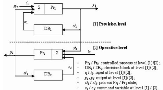
Fig. 4. Two-loop control model for the Operational control
