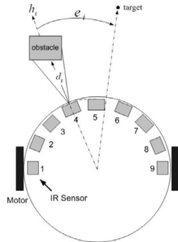
Fig. 2. Fuzzy linguistic variables  $d_i$  which is the distance of the obstacle measured by  $i$ th sensor and  $e_i$  which is the angle from  $h_i$  to a target.
