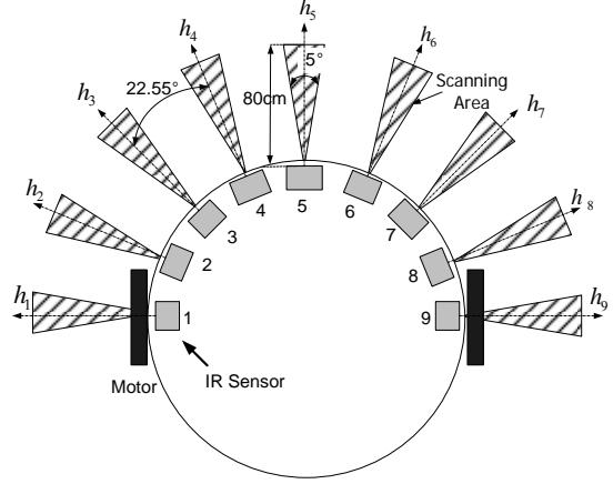
Fig. 1. Mobile robot model and definition of heading directions  $h_i$ ,  $i=\{1,2,\dots,9\}$ .
