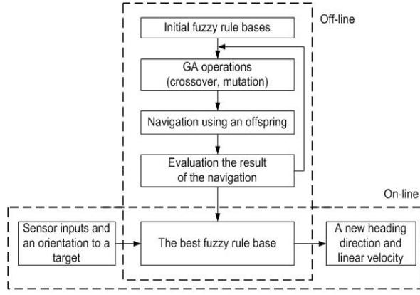
Fig. 4 Proposed off-line and on-line processes
