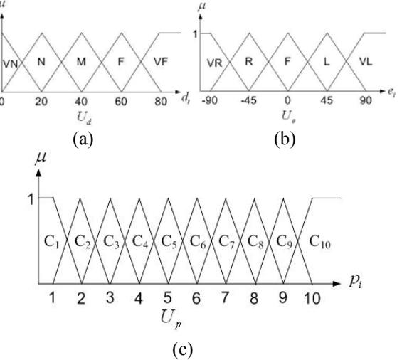
Fig. 3 Membership functions of measured distance  $d_i$
