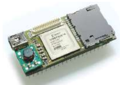
Fig. 8. Virtex 4 FPGA used to implement the system-on-chip for the central controller
