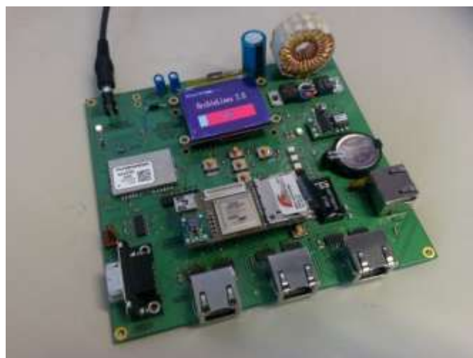
Fig. 9. Central controller board
