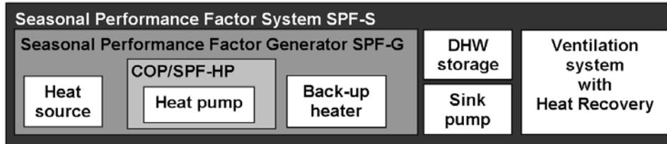
Figure 3: System boundaries for the assessment of the monitored compact unit
