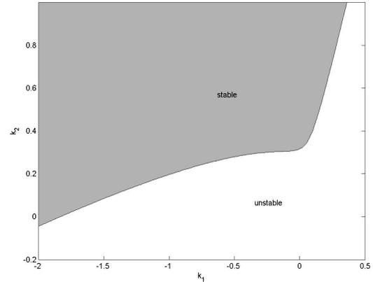
Fig. 2. SOF example HE11. Region of stabilizing gains (in gray).
