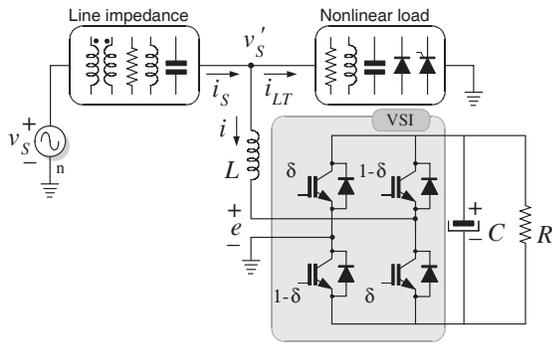
Fig. 1. Single-phase full-bridge shunt active filter connected to a distribution system.
