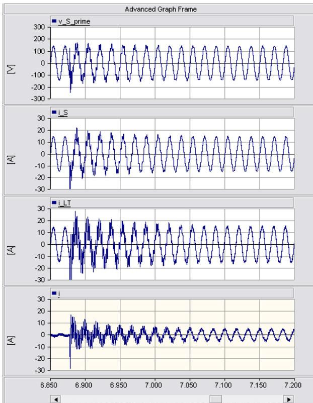
Fig. 7. Transient responses, under the proposed compensator of Fig. 5, during the connection of capacitor  $C_L$  on the load side of: **(from top to bottom)** line voltage  $v'_S$ , compensated line current  $i_s$ , load current  $i_L$  and active filter current  $i$ .
