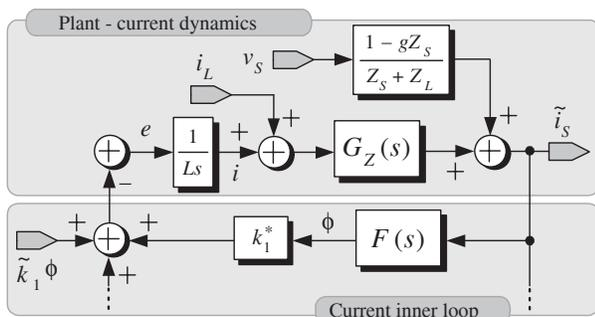
Fig. 4. Block diagram of the modified current loop.
