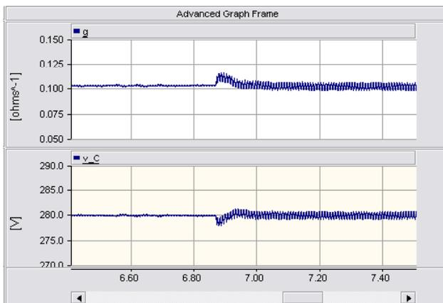
Fig. 8. Transient responses under the proposed controller when capacitor  $C_L$  is connected on the load side: **(top)** the equivalent conductance  $g$  and **(bottom)** the capacitor voltage  $v_C$ .
