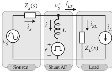
Fig. 2. Equivalent circuit of a shunt active filter connected to a more realistic distribution system considering load and line impedances.
