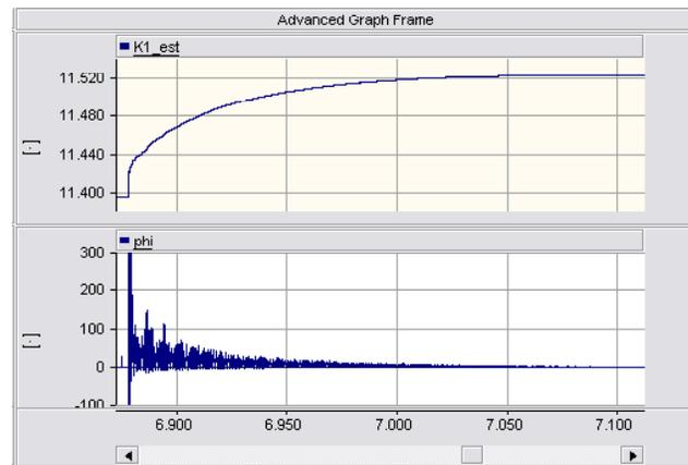
Fig. 9. Transient responses under the proposed controller when capacitor  $C_L$  is connected on the load side: **(top)** the estimated damping term  $k_1$  and **(bottom)** the regressor  $\phi$ .
