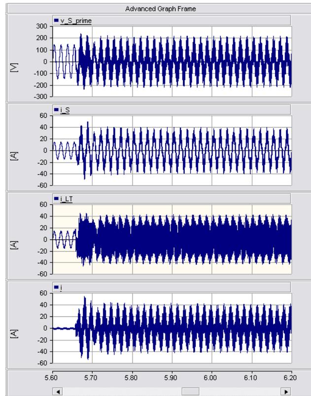
Fig. 6. Transient responses, under the original compensator (5) and (7), during the connection of capacitor  $C_L$  on the load side of: (from top to bottom) line voltage  $v'_S$ , compensated line current  $i_S$ , load current  $i_L$  and active filter current  $i$ .
