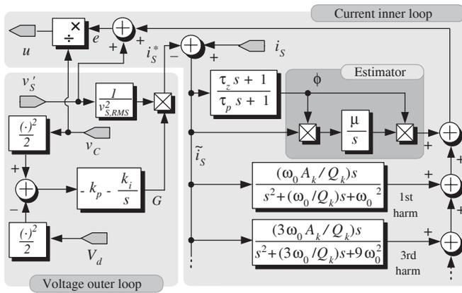
Fig. 5. Block diagram of the overall proposed controller.
