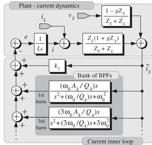
Fig. 3. Block diagram of the current loop considering load and line impedances.
