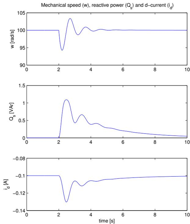
Fig. 3. Simulation results: Mechanical speed, reactive power and  $i_d$  current, for a change of the external torque.
