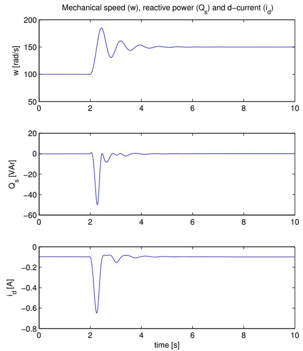
Fig. 2. Simulation results: Mechanical speed, reactive power and  $i_d$  current, for a change of the speed reference.
