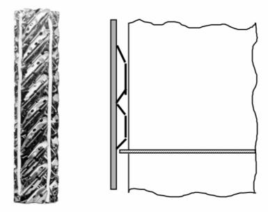
Figure 7: Wall bypassing: Teflon gaskets for pilot size / double mode wall vipers for industrial size
